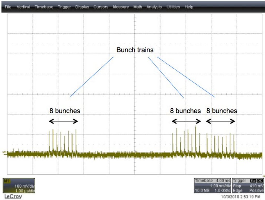
Figure 28: Zoom 10^3 (1 \mu s/div): The bunch-train structure shows 8 bunches per bunch train. On the left side there is one train and on the right side there are two consecutive trains.
