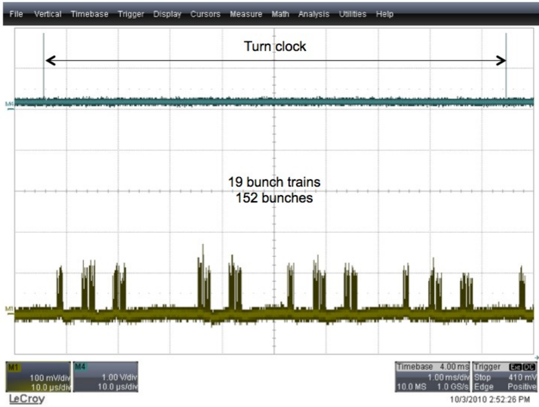
Figure 27: Zoom factor 10^2 (10 \mu s/div): The bunch-train structure shows 8x16 and 3x8 bunch trains, corresponding to 152 bunches.
