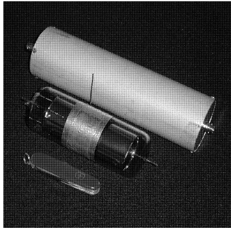
Figure 2. FNAL 110\text{-cm}^3 sealed-glass argon ionization chamber and its container.
