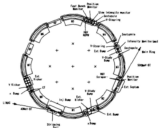
Fig.4 Plan of the KEK-PS-Booster ring
