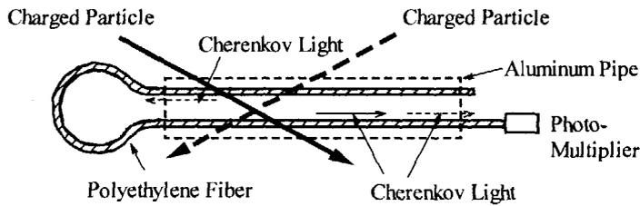
Fig.8 How to set the photo-fiber for removing the position effect of the photo-multiplier
