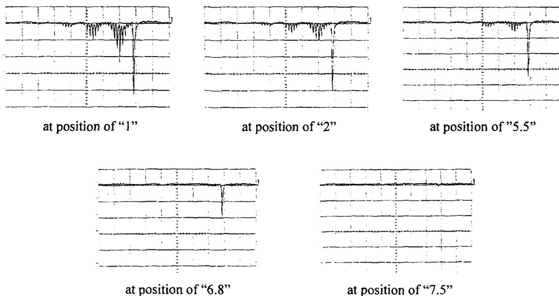
Fig.7b Beam loss at extraction observed by lower loss monitor (x:1 $\mu$ s/d)
