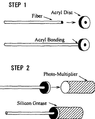
Fig.1 Method used to connect a photo-fiber to a photo-multiplier
