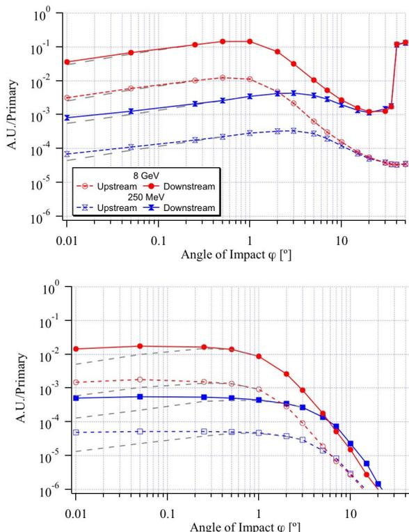
Figure 2: Fiber responses per primary electron as a function of  $\varphi$  the impact angle of the electron beam for a fiber located just above the point of impact ( $\theta = 90^\circ$ , top) and opposite ( $\theta = -90^\circ$ , bottom). The grey dotted lines are for the responses measured within  $\pm 1$  m of the point of impact.
