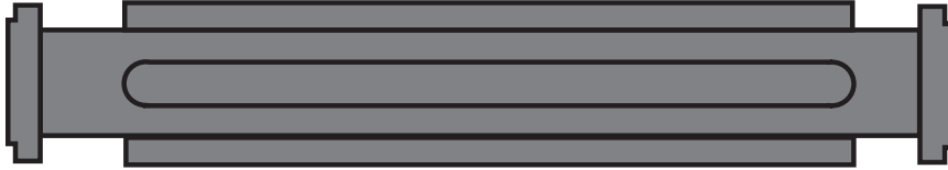
Figure 5.21: Side view of the titanium magnet form on which the racetrack coils fit.
