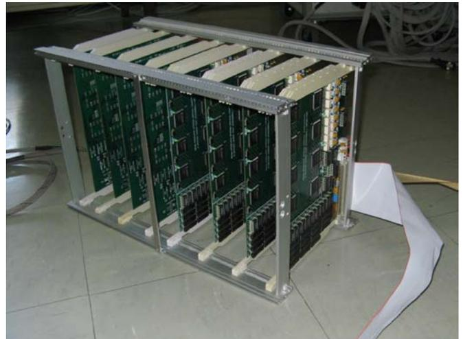
Fig. 6: Experimental test setup for the 2x32 CPLD devices from Xilinx. The DUTs are the XC95144 operating at 5.0 V and the XC95288XL operating at a bias voltage of 3.3. V.
