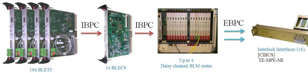
**Figure 2.** The Internal Beam Permit Check (IBPC) tests the beam permit links of the BLM system; the External Beam Permit Check (EBPC) tests the connections from the BLM to the interlock system.
