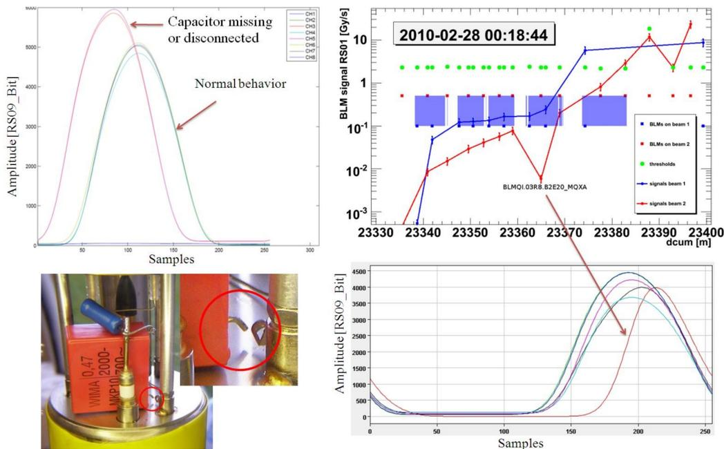
**Figure 5.** Modulated signal (left-top) with a non-conformity on the HV input filter shown on the detector (left-bottom). Detector sensitivity loss due to non-conformity of the tunnel card discovered by measurements with beam (right-top) and confirmed by the connectivity check (right-bottom).
