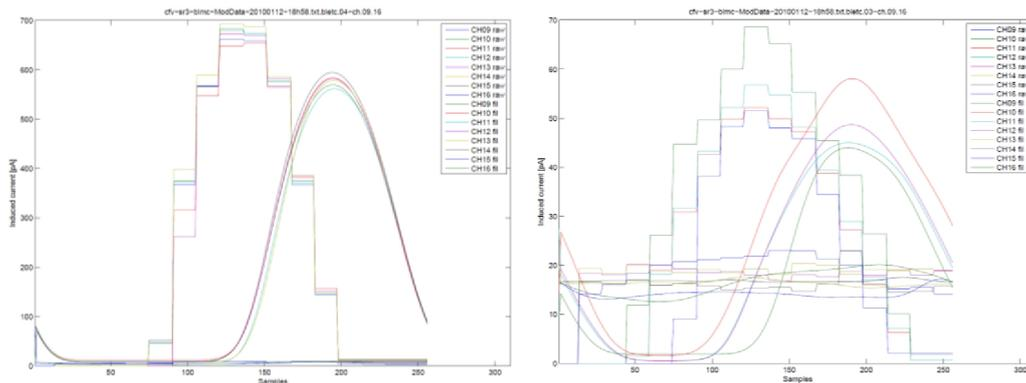
**Figure 3.** Volatile memory data for IC (left) and SEM (right). The raw data received from the CPU (stairs) are smoothed by a low pass filter (FIR) before amplitude and phase determination.
