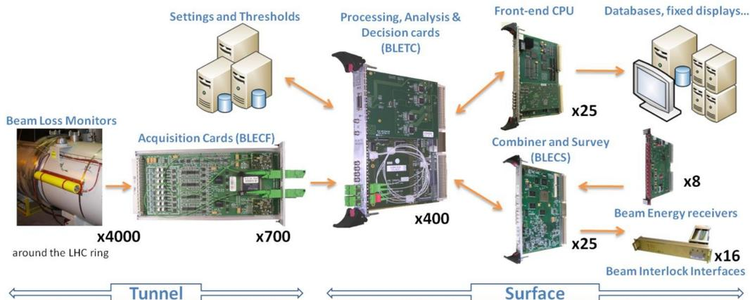
**Figure 1.** Overview of the LHC BLM hardware system.
