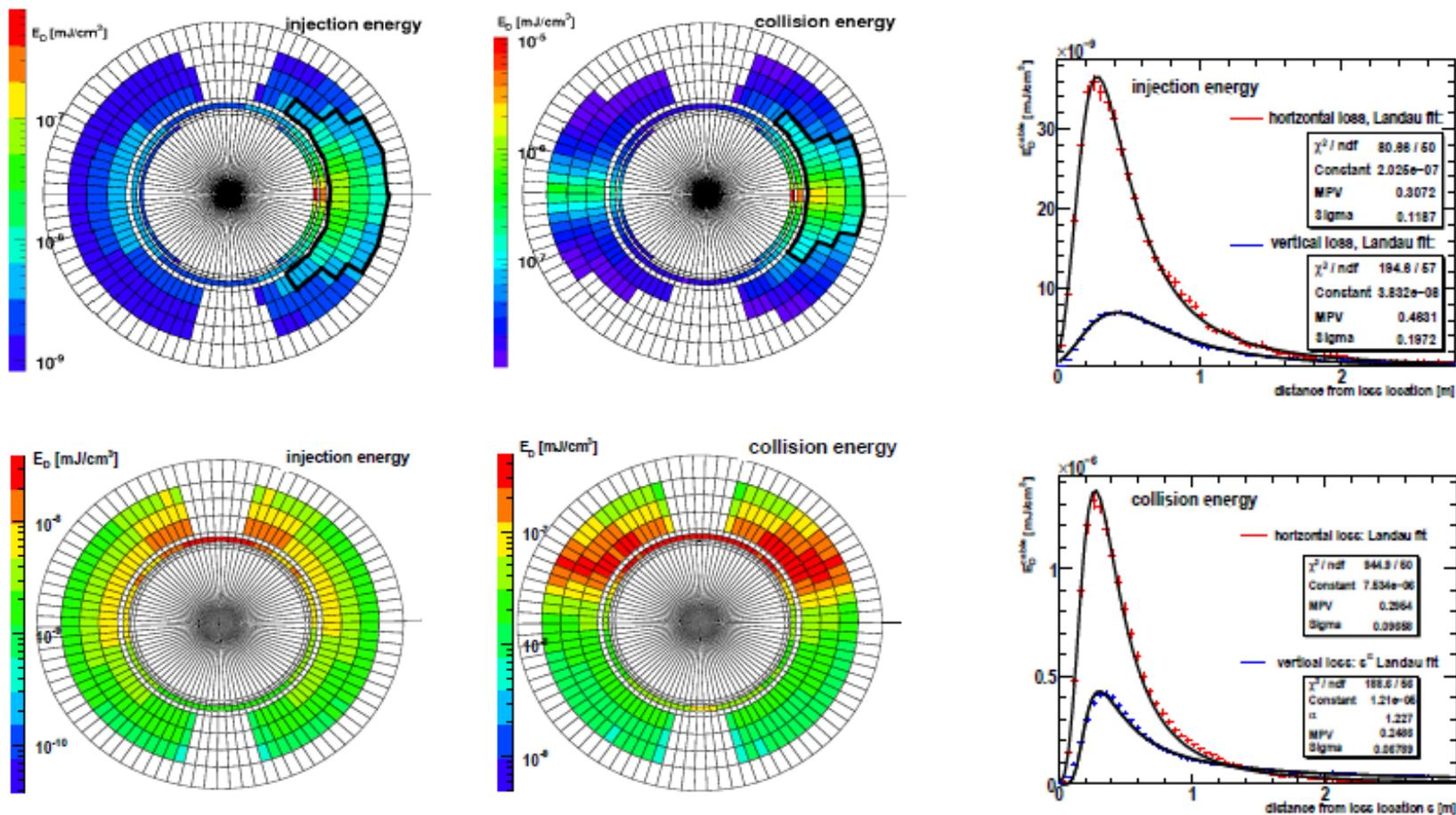
Figure 9: Energy density distribution per impacting proton for the most exposed azimuth in the thermal equilibrium volume of the inner coil. The shape of the distribution is the same as in case of  $E_D^{\max}$ .
