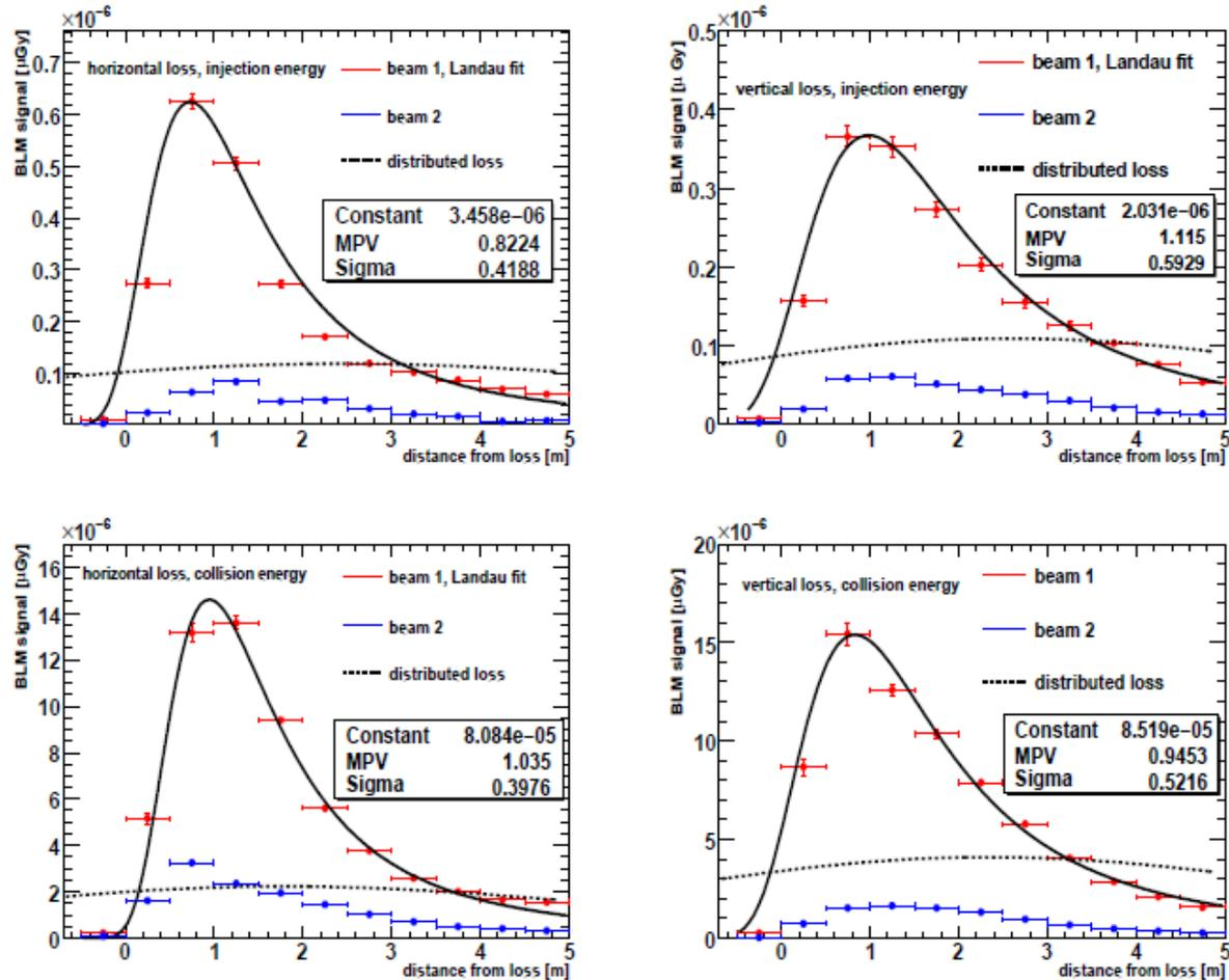
Figure 17: Signal per impacting proton in BLM cylinders along the cryostat as a function of distance from the loss location. Left upper plot: injection beam, horizontal loss (outwards the magnet center). Right upper plot: injection beam, vertical loss. Row below: for collision energy.
