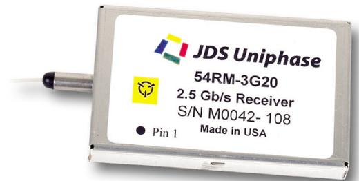
The JDS Uniphase 54RM series receiver module is designed for use in telecommunications systems and high speed data communications applications. It is optimized for SONET OC-48 and synchronous digital hierarchy (SDH) STM-16 line interfaces. Its uniform package, pin function, and common optical and electrical characteristics are multisource agreement (MSA) compliant.
