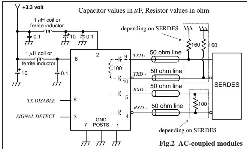
Fig.2 AC-coupled modules
