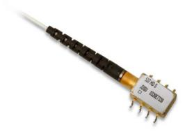
The JDS Uniphase ERM 537/547 series consists of small form factor (SFF) 2.5 Gb/s SONET/ SDH optical receivers with InGaAs PIN or avalanche photodiodes and high bandwidth linear transimpedance amplifiers. They are available with differential outputs. The differential outputs can be used for added gain or for signal monitoring.
