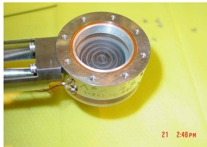
Typical Faraday Cup (energy degrader removed)
