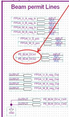
We can see also the inputs from the crates (FPGA\_x\_x\_neg\_In) for Unmaskable (U) and Maskable (M) with redundancy (A and B)
