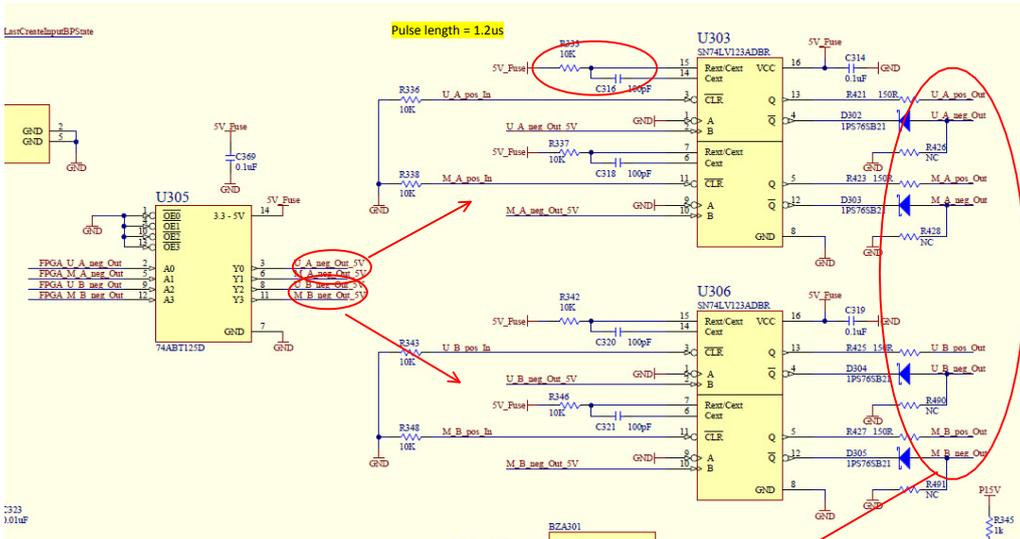
The output lines (positive and negative, U and M, A and B) are then routed to the connector P2 user assignable lines (free lines specified in the VME64 standard).
