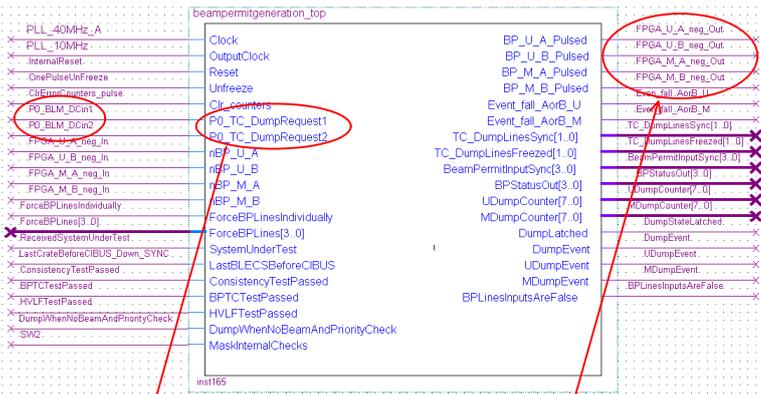
Inside this block, each "BeamPermitControlCell" is assigned to take care of one signal (U or M and A or B). The signal from the BLETC is splitted at this level between the redundant block A and B
