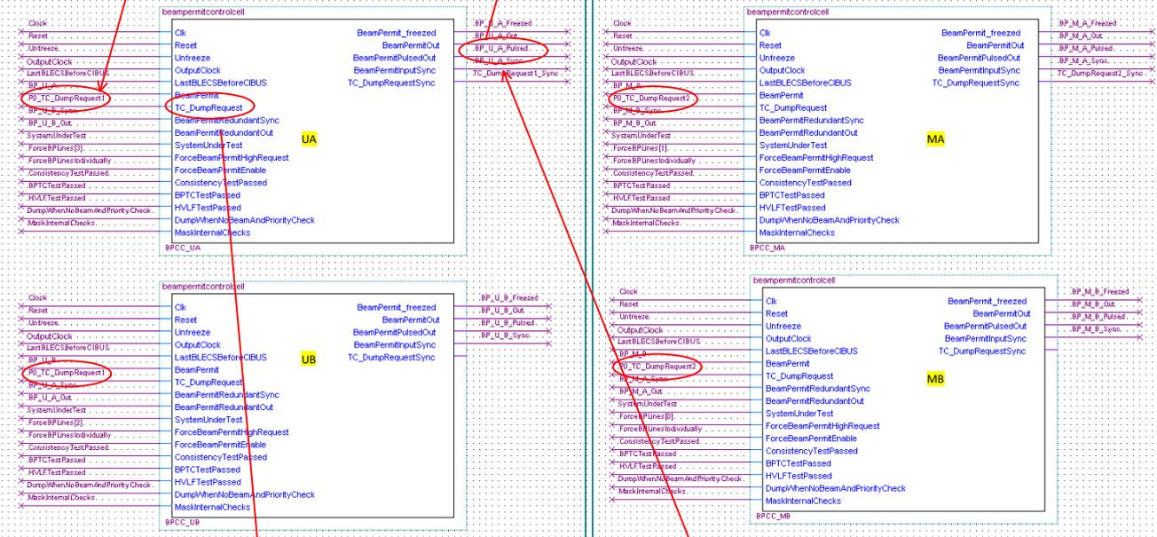
Inside each of the block the combination is done: After being synchronized, the beam permit signal from the BLETC (TC\_DumpRequest) is combined with other signal (including the signal from other crates "BeamPermit") to generate the final signal "BeamPermitCombined". This signal controls the generation of the frequency. This frequency leaves the FPGA.
