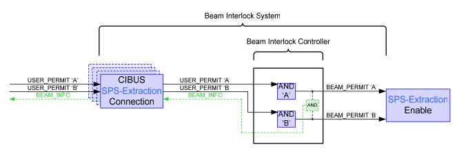
Figure 3: Simplified Architecture of SPS Extraction and Transfer Lines Interlock System
