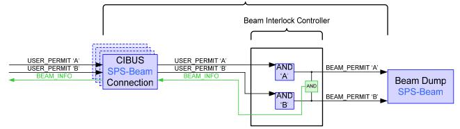
Figure 2: Simplified Internal Architecture of the SPS Beam Interlock System
