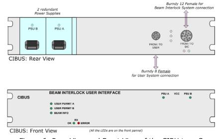
Figure 6: Rear View and Front View of the CIBU type S
