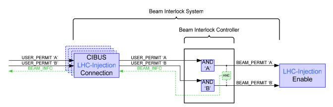
Figure 4 : Simplified Internal Architecture of the LHC Injection Interlock system
