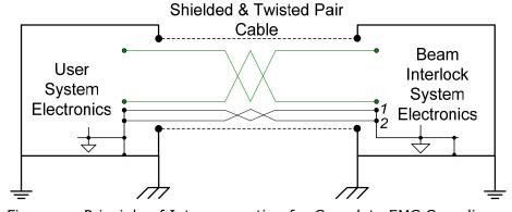
Figure 12: Principle of Interconnection for Complete EMC Compliance
