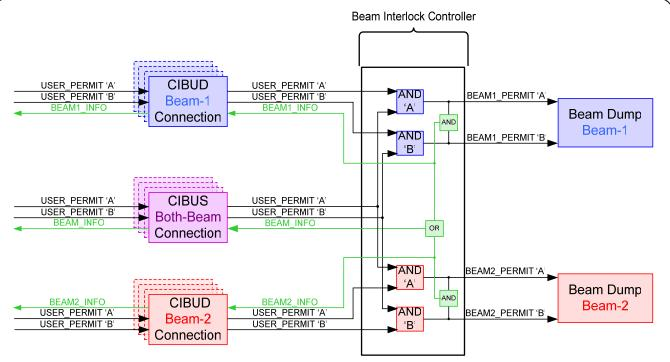
Figure 1: Simplified Internal Architecture of the LHC Beam Interlock System
