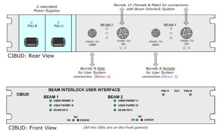
Figure 5: Rear View and Front View of the CIBU type D
