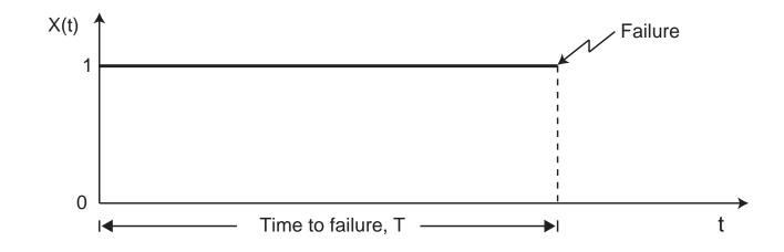
$X(t) = \begin{cases} 1 & \text{if the item is functioning at time } t \\ 0 & \text{if the item is in a failed state at time } t \end{cases}$
