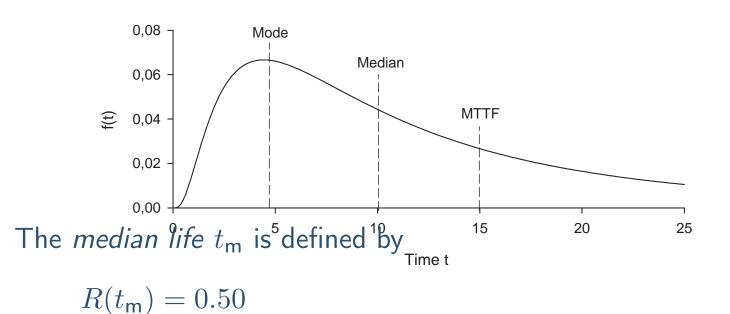
The median divides the distribution in two halves. The item will fail before time  $t_m$  with 50% probability, and will fail after time  $t_m$  with 50% probability.
