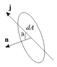
Here,  $\mathcal{G}$  is the angle between  $\mathbf{j}$  and  $\mathbf{n}$ This holds for any dA in any direction Also, it is positive if more neutrons are crossing in the  $+\mathbf{n}$  direction and negative if more neutrons are crossing in the  $-\mathbf{n}$ direction
