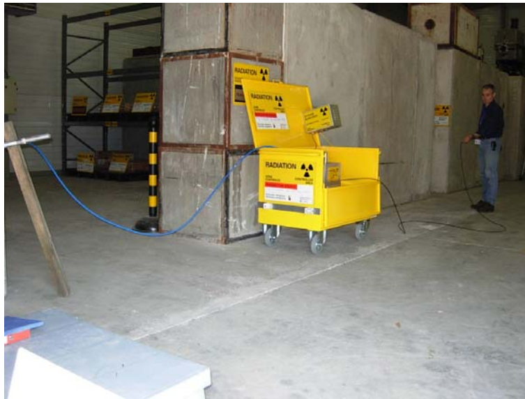
Figure 1 Demonstration of irradiation procedure. The source clamp is on the left side and the operating person is on the right side, keeping the distance in between maximal.
