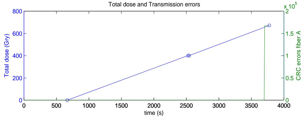
The errors stated on fiber channel, then the second soon after (5s). 15 seconds later the crc errors become lose of frames. (complete loss of the signal)
