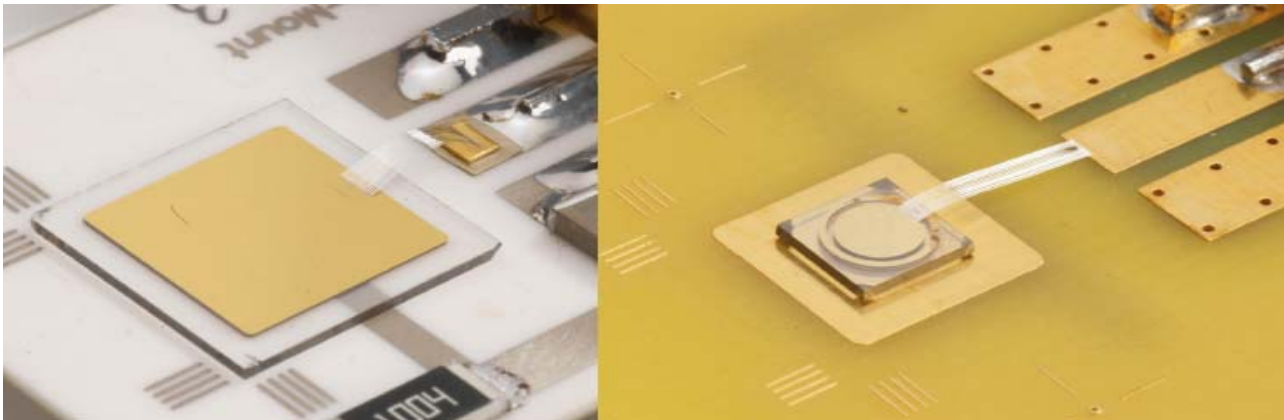
Figure 1: Single-crystalline and poly-crystalline diamond substrates, metalized with gold, are mounted on a ceramics board and a FR72 board, respectively.
