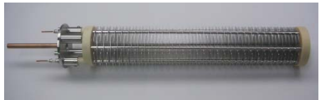
Fig. 2. Inside structure of the LHC BLM (ionization chamber).
