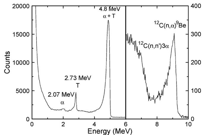
Fig. 3. PHS recorded with a  $^6\text{LiF}$  "sandwich" detector. The reaction with 14 MeV neutrons is evidenced in the right side.
