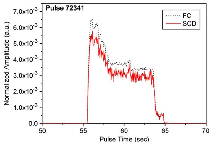
Fig. 7. Time dependent neutron emission during JET pulse #72341 recorded by Det-3 coupled to DBA and compared with one of the Fission Chambers routinely operating at JET.
