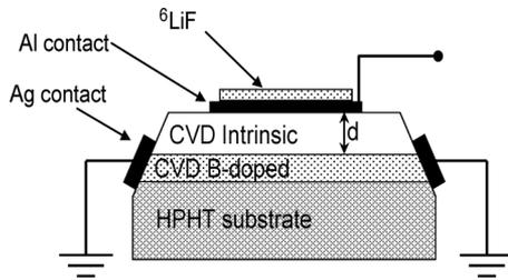
Fig. 1. Layered structure for the SCD detector.
