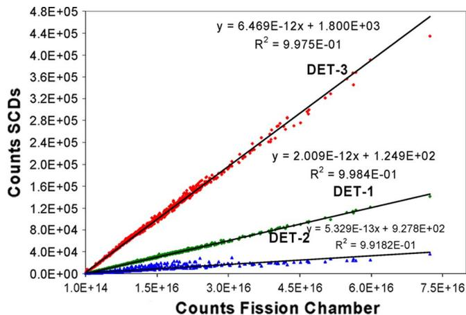
Fig. 5. Correlation among SCD detectors and Fission chamber at JET tokamak (results March–April 2008).
