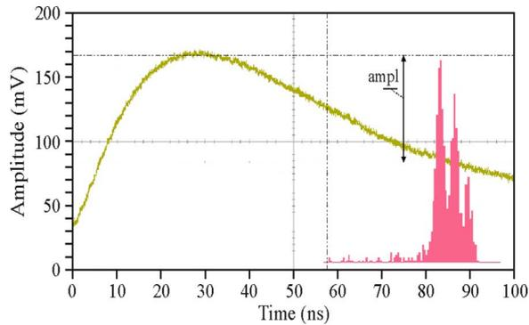
Fig. 8. PHS (histogram) as recorded by oscilloscope for the three alpha peaks source ( $^{240}\text{Pu}$  (5.3 MeV) +  $^{241}\text{Am}$  (5.5 MeV) +  $^{244}\text{Cm}$  (5.8 MeV)) by using the FCA developed in this work. The output pulse is also shown.
