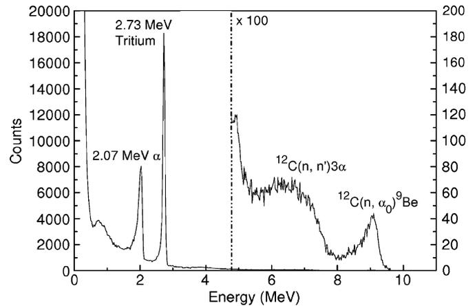
Fig. 2. A typical PHS measured with a LiDia Detector irradiated in a PMMA phantom with 14 MeV neutrons.
