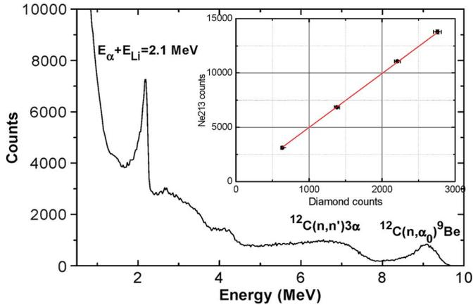
Fig. 4. a) PHS for Boron sandwich detector. The single peak is clearly evidenced. b) The inset shows the detector linearity tested versus NE-213 scintillator.
