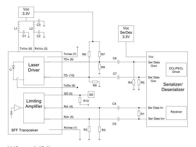
$\begin{array}{lll} \text{L1, L2:} & 1...4.7 \ \mu\text{H} \\ \text{C1, C2, C3:} & 4.7...10 \ \mu\text{F} \\ \text{C4, C5, C6, C7:} 100 \ n\text{F} \\ \text{R1:} & 100 \ \text{Ohms} \\ \text{R2, R3:} & 150 \ \text{Ohms} \end{array}$
