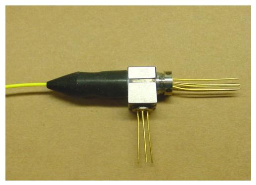
These small, compact modules require minimal board real estate and when used in pairs deliver full duplex operation of a single 9/125um optical fiber. The use of high performance optical filters maintains an optical cross talk between the channesl <-24dB.
