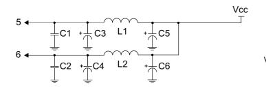
Values C1/C2= 100nF Ceramic C3/C4/C5/C6= 10uF Tantal L1/L2=3.3uH Coil or Ferrite Inductor
