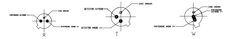
PD-LD aligns then secures each TO-Packaged photodiode within a universal alignement sleeve. This assembly may then be incorporated into a connector receptacle assembly (FC, SC, ST, ect) or into a fiber pigtailed assembly. Some examples of housings are listed here, but other packages are available upon request, including board mountable SC and FC styles. The standard pin-out rotation is to have the TO can tab at 1:00 when the assembly is viewed from the rear and the key slot is up (12:00).
