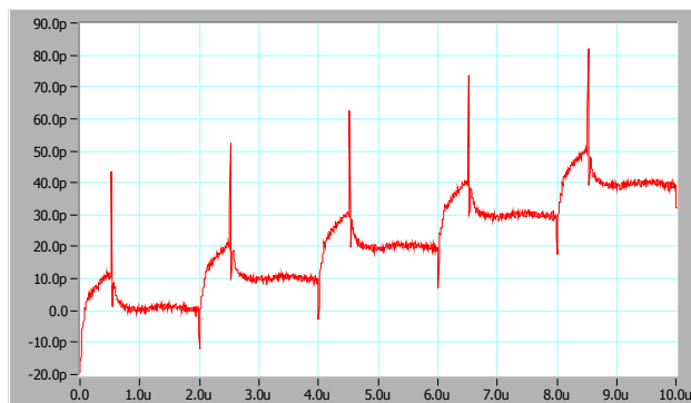
Figure 4: ~9.8pC steps for 2µs spacing
