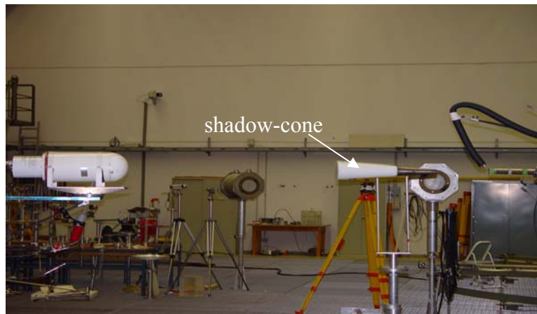
Figure 10 Measurement setup with a shadow-cone placed between the target and the chamber to determine the contribution of scattered neutrons to the recorded signal.
