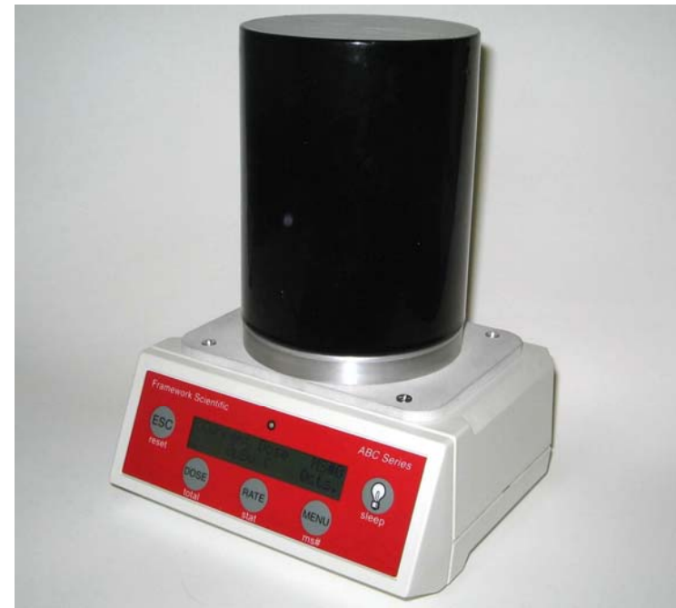
Acoustical bubble counters, open and with lead shell (F. d'Errico, University of Pisa)
