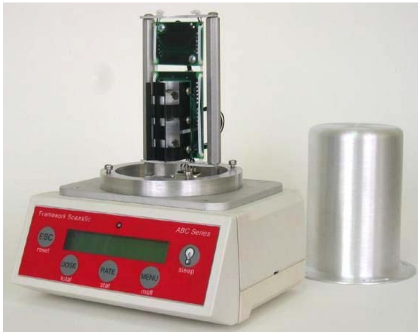
Acoustical bubble counters, open and with lead shell (F. d'Errico, University of Pisa)
