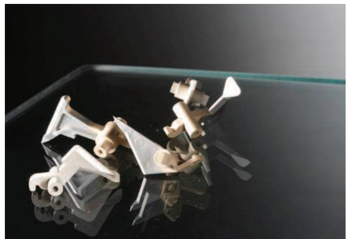
VICTREX® HT™ polymer replaced metal with fluoropolymer coatings in printer split finger eliminating the need for secondary processing providing high temperature performance in a tribological environment.
