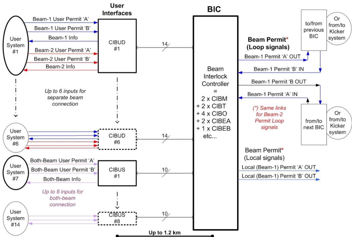
Fig.2: In the LHC case, the BIS manages two beams: dedicated *User Interfaces* are available for double connection (type CIBUD) and the corresponding signals are dual.
