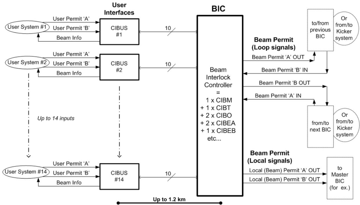
Fig.1: For most of the Beam Interlock Systems, the *Beam Interlock Controller* and the distant *User Interfaces* (type CIBUS) are composing the hardware solution
