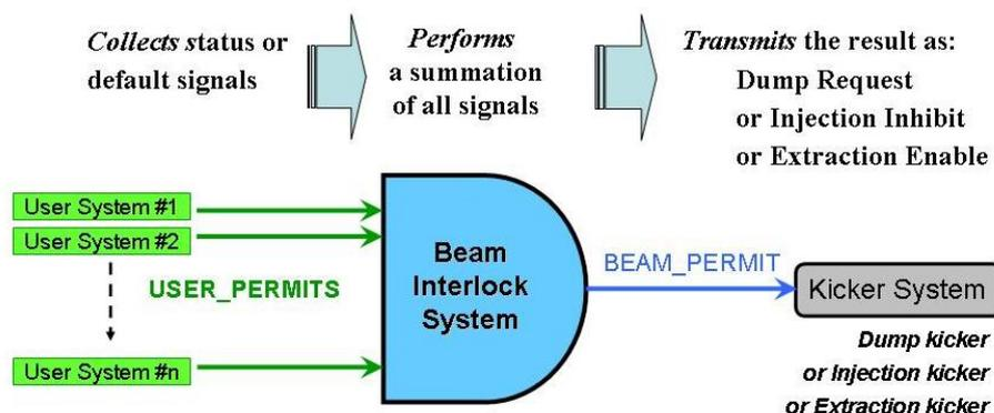
In all cases, the same hardware solution is used with a central element called the *Beam Interlock Controller (BIC)* and distant elements called the *Beam Interlock User Interfaces* (see Figures in Appendix#1)
