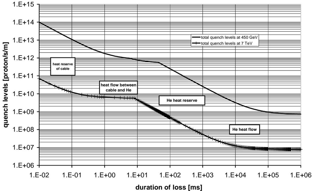
**FIGURE 2.** Calculated quench level for LHC dipole.
