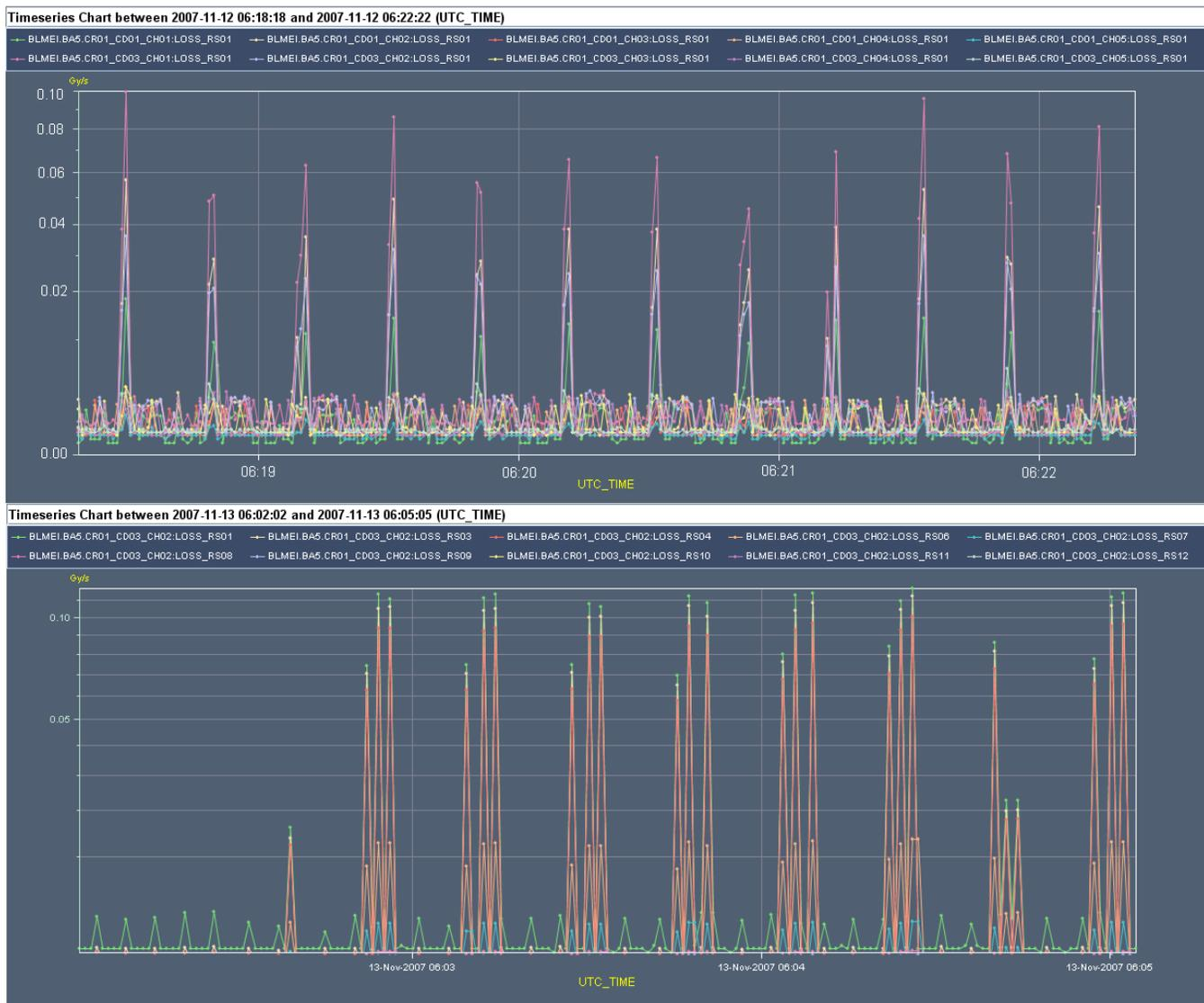
Fig. 1: Losses (Gy/s) recorded in the Logging database during the 2007 ‘Machine Development’ test in the SPS accelerator. They have been plotted using the TIMBER tools provided for the extraction of data from the database. [top] Plot of the 40  $\mu$ s integrals from different Ionisation Chamber channels showing occurring losses at the beam injection. [bottom] Plot of ten integrals (spanning from 40  $\mu$ s to 84 s) from the same Ionisation Chamber channel showing losses at the collimator.
