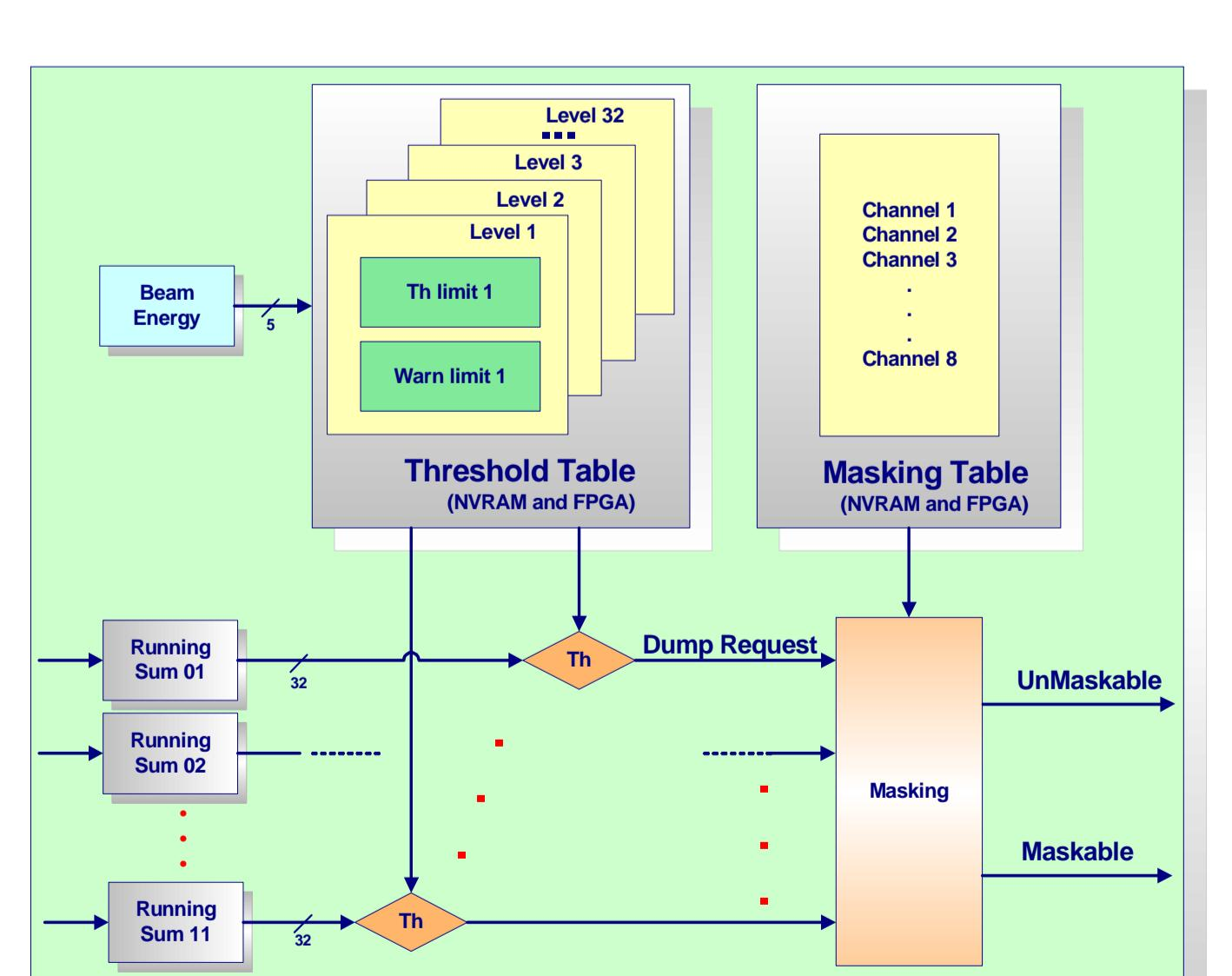
The tables are stored on the *BLM Mezzanine*'s non-volatile memory and can be unique for each detector.
