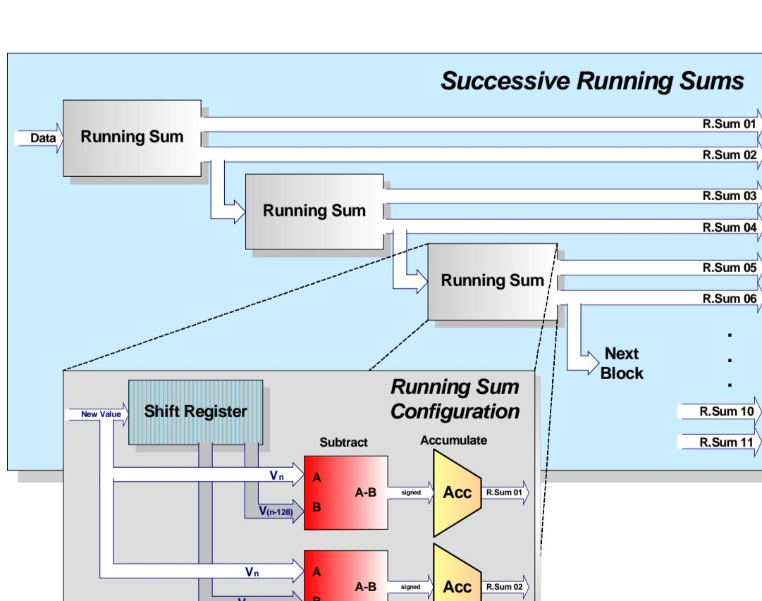
the multipoint shift registers available on the *Stratix* devices and it is adding the difference of those two values to an *Accumulator*.
