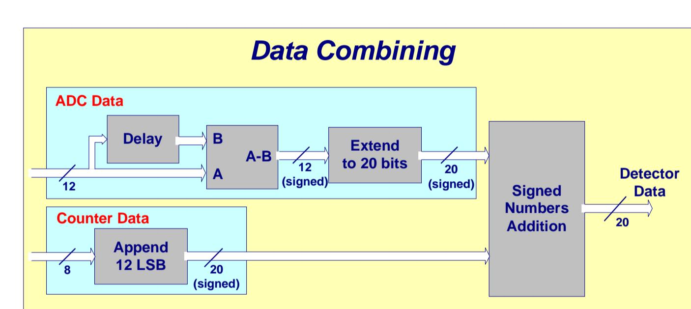
Based on the fact that the two types of data acquired for each detector are different, a pre-processing is needed in order those to be combined seamlessly.
