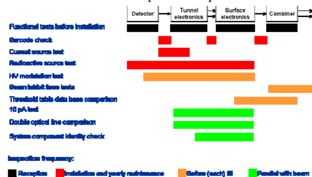
Figure 14: Schematic of test for the LHC beam loss system.
