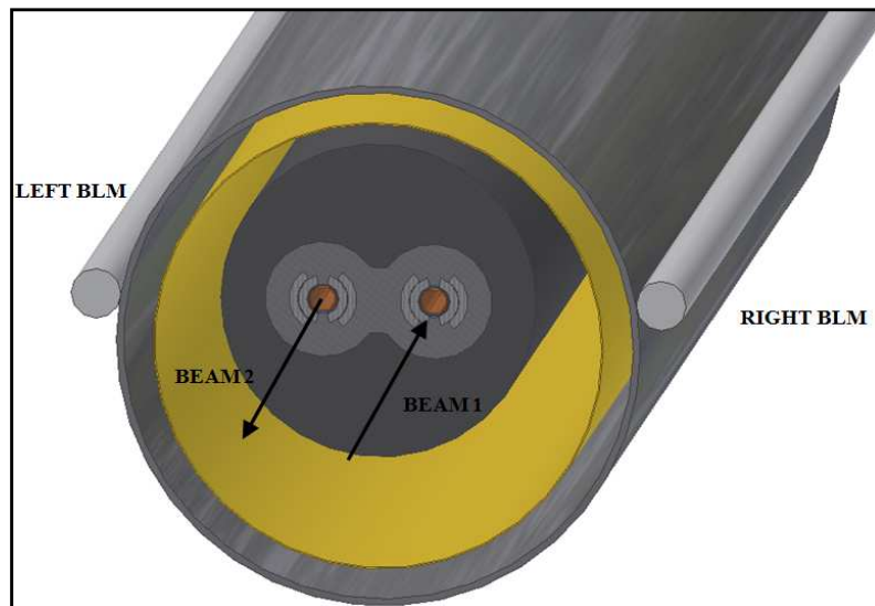
Fig.6.1.1: Two detectors record secondary particles coming from the clockwise beam and the counter-clockwise beam. Originally the right BLM surveys the beam 1 and left BLM observes beam 2 but the cross-talk also occurs.
