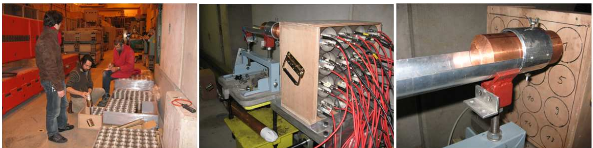
Fig.3.4.4: Testing the Secondary Emission Monitors (SEM). Description in the text.
