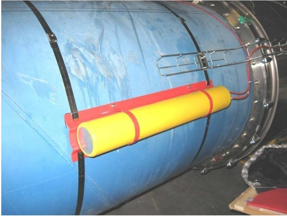
Fig. 3.4.3: All LHC BLMs are painted yellow. One the picture: BLM mounted on Main Dipole.
