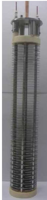
Fig. 3.4.2: Picture of the LHC BLM detector without the cover tube [7].
